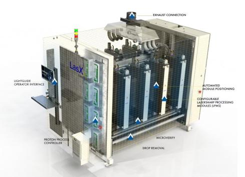
FreshFocus uses standardized components, adding a higher guarantee of performance and consistency to your converting process.
