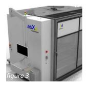
**MicroVerify:** LasX is introducing an affordable, high-speed, inline inspection system for quality assurance for the small laser holes and score lines that are produced. MicroVerify provides instant feedback and alarms that can be configured for specific warning thresholds.
